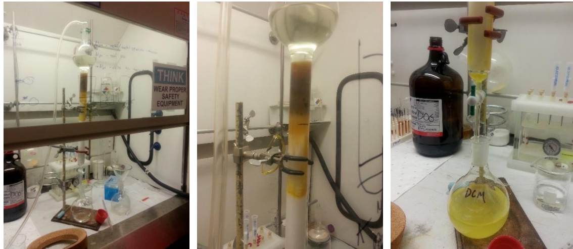
Figure 4.1 Images of the reservoir column packed with Iatrobeds in the body of the column and the plug of metabolites at the top. Dichloromethane is being pushed through in these photos.
